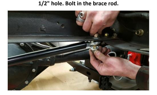
Now you can bolt in the new panhard rod. This has a RH and a LH rod end. The hex end of the bar has RH threads. This makes adjustment easier without needing to unbolt the bar to adjust the rear axle center. To start with try the center hole on the Chassis side and the top hole on the trailing arm side. Once the bed is back on you can set the bar. The goal is to try to keep it a level as possible for neutral handling.
