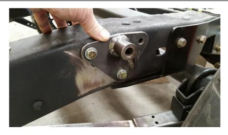
Now it's drill time. Use a 3/8" drill to drill out the rear hole for mounting the coil-over bracket. Then use a 5/8" bit to drill through the frame for the upper coil-over mount bolt. Put the third mount bolt in place.
