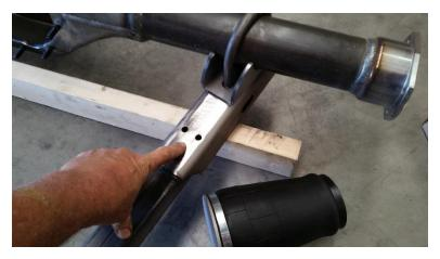
18. The upper bag mount plate will weld to the Boxing plate on the inside of the frame rail. For now, just tack the bracket in place.
