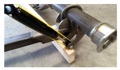
20. It can be mounted "In and Back" (I prefer "Out and Forward" as it has less interference with the panhard rod) the top shock mount is a simple tube welded to the top of the frame. The shocks can be tilted forward or back up to 30 degrees, which will allow for more axle travel.
