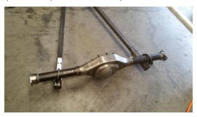
12. Carefully move the axle side-to-side until it is centered. Measure each side from the trailing arm to the axle end. – Did you see the arm move? Oh Snap!
