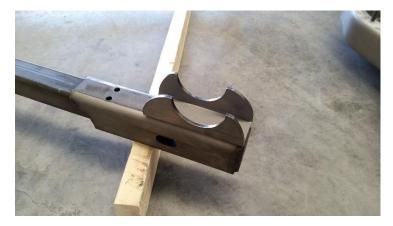
11. Then, set the axle in place and drop in the U-bolts to help locate the saddles.
