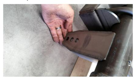
22. The upper mount is a crossmember that spans from boxing plate to boxing plate. Shown here resting on the top of the housing. We recommend that you place the crossmember "Behind" the shocks, to give the axle housing more room. To help position the crossmember, bolt the shocks in place to the lower mounts —with no springs, drop the axle 2" to 2 ½" from ride height, then bolt the tops of the shocks to the crossmember. Fit and tack the crossmember in place.
