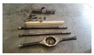
2. Bolt the brackets to the front crossmember. I use only two bolts on each here to save time, but that's just me. Yes, the pivot bolts will run up and down.
