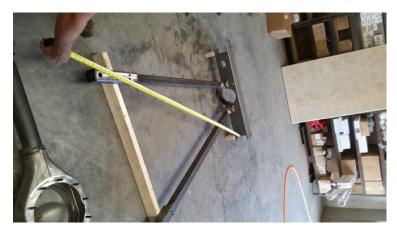
9. (C) Now measure from the crossmember back to the tip of the trailing arms as shown. Check both sides. If they aren't the same, start over at step #3. If they are, you one step closer to being a real Hot Rodder, and you can move on to the next step.
