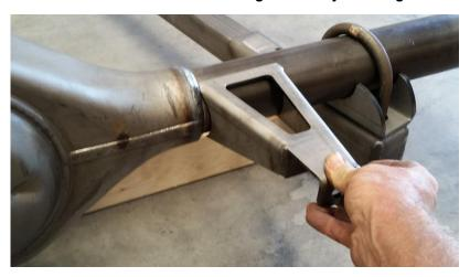
24. Looking down, the panhard rod may tip "back" to clear the coil-over shocks. That's OK. Looking at the bar from the back, try to keep it level at Ride Height. You may need to fabricate a small spacer for the chassis side mount to do this, depending on the chosen ride height.
