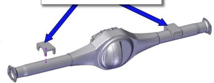
axle sitting all the way into these mounts and CRITICAL to center the axle on both sides.
