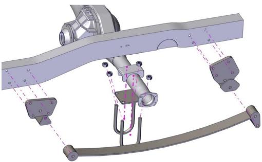
• Chisel, torch, drill, or press out the rivets that hold the leaf spring mounts and shackle hangers onto the frame, however you need to just get them off and throw that junk in the trash.
