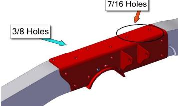
•Only install the 3/8" Hardware, the 7/16" hardware will be needed in a later step. Use the C-Notch Hardware bag for this install.
